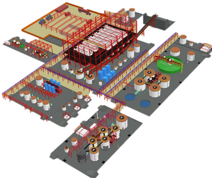
Figure 6 - 3D FEED layout of concentrate processing facility
