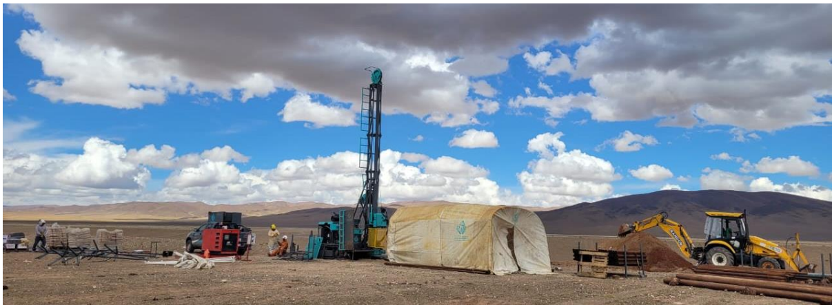
Figure 1. Drill rig at Jam 24-01 with 800m drill rods stored to right. A 30m steel pipe is cemented at top of the well. The rig is triple tube HQ diameter. The anticipated depth is 400m.
