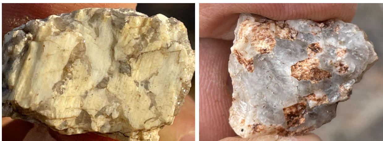
Figure 4 - Example of weakly weathered pegmatite drill chips observed in historic RAB drill hole JBR296 (left), and strongly weathered pegmatite from historic drill hole JBR140 (right) 6
