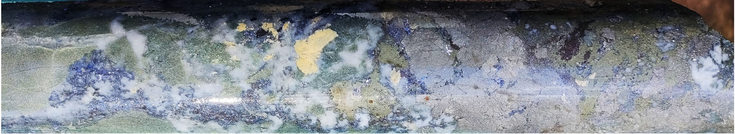
Hornfelsed Mathinna Sediment host - Quartz vein with pyrite-arsenopyrite-pyrrhotite-galena-sphalerite and hornfelsed clasts in TFDD005 at 120.3m (0.7m @ 152.5g/t Au)
