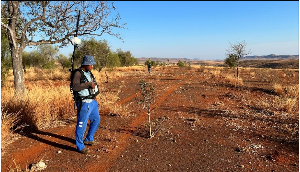
Appendix Figure 2. Photographs of (a) the surveying team (b) the southern survey area (25m survey line spacing) looking south (c) the survey walker in foreground preparing to start ground magnetic surveys.
