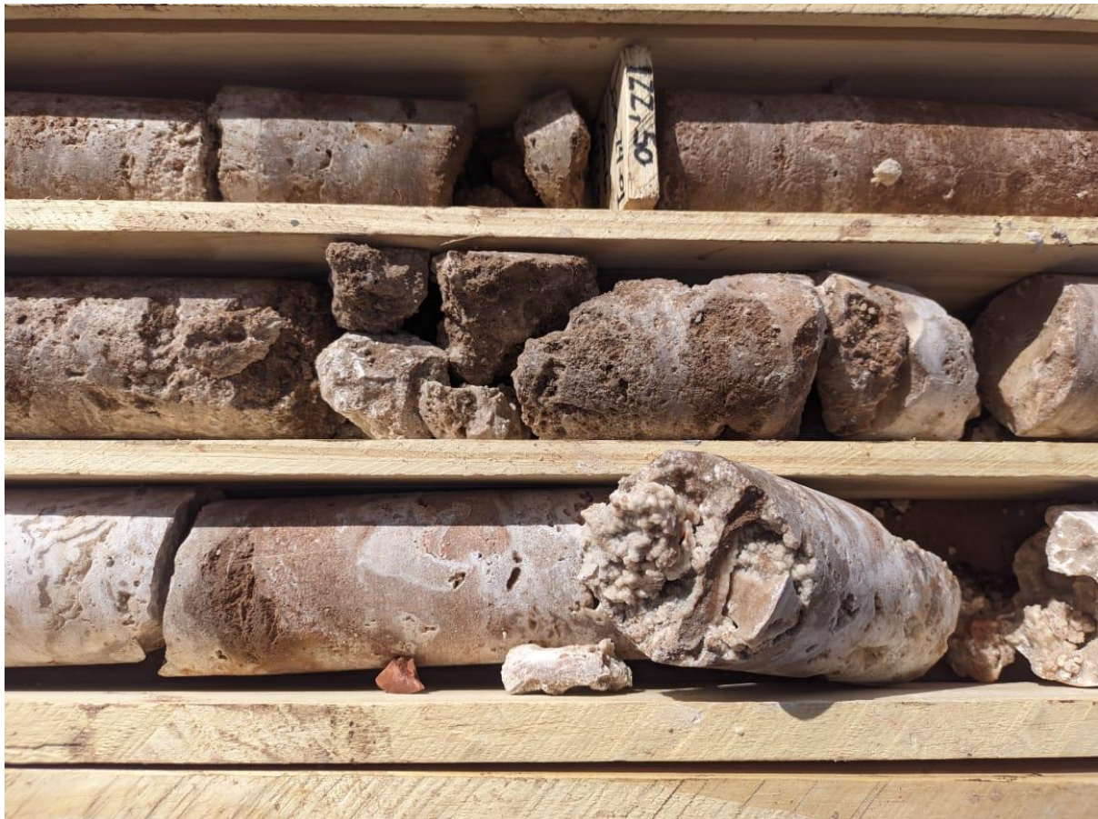
Figure 4. Porous calcareous units with macropores at 122.50m depth indicative of an aquifer zone with secondary mineralisation indicating evaporites are present concentrating minerals.
