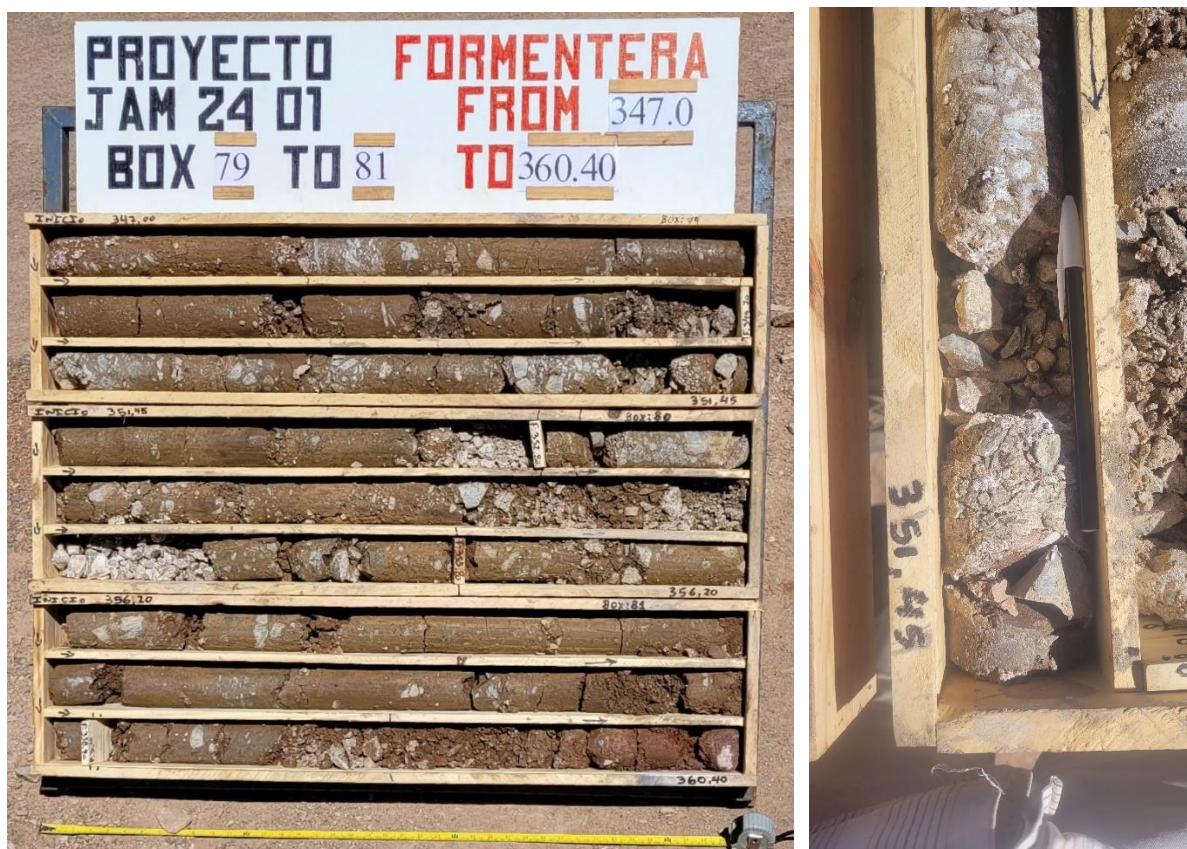
Figure 2. Gravel sequence from 347m to 360m with exceptionally high porosity allowing brines to flow.
