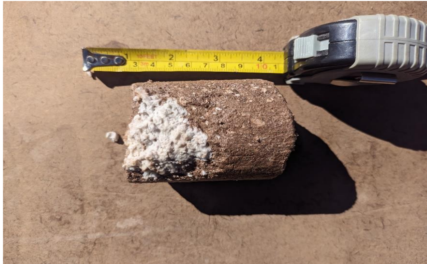
Figure 1. Borate crystals in drill core at 270m depth – indicating presence of boron which is often associated with lithium deposits. Boron forms in small pillow shaped crystal masses.
