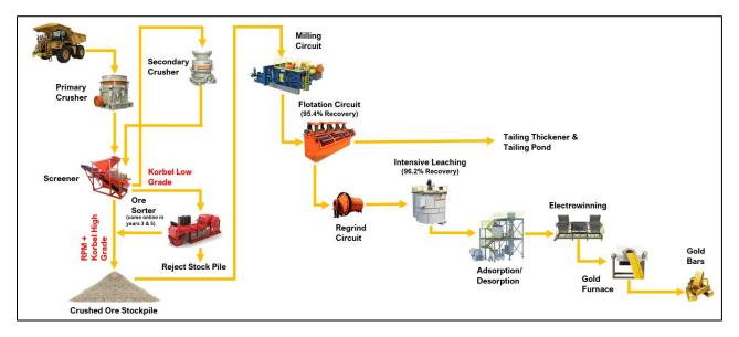
Figure 14-1: Simplified process flow sheet
