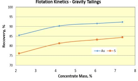
**Flotation Kinetics - Gravity Tailings**
