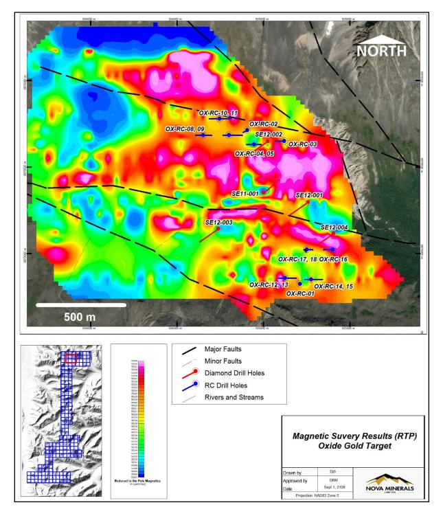
Figure 7-4: Magnetic Survey Results (RTP)
