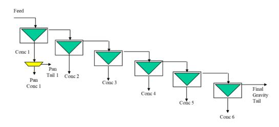
Figure 10-1: GAT test flowchart
