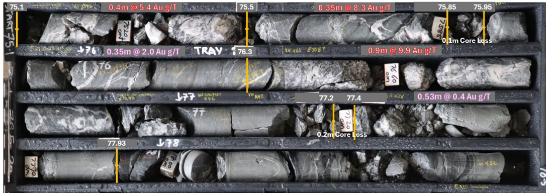
Photographed core from DNDD001 showing high grade gold intervals in lode style quartz veins from mineralised zone 7.2m @ 2.5g/t Au from 68.9m
