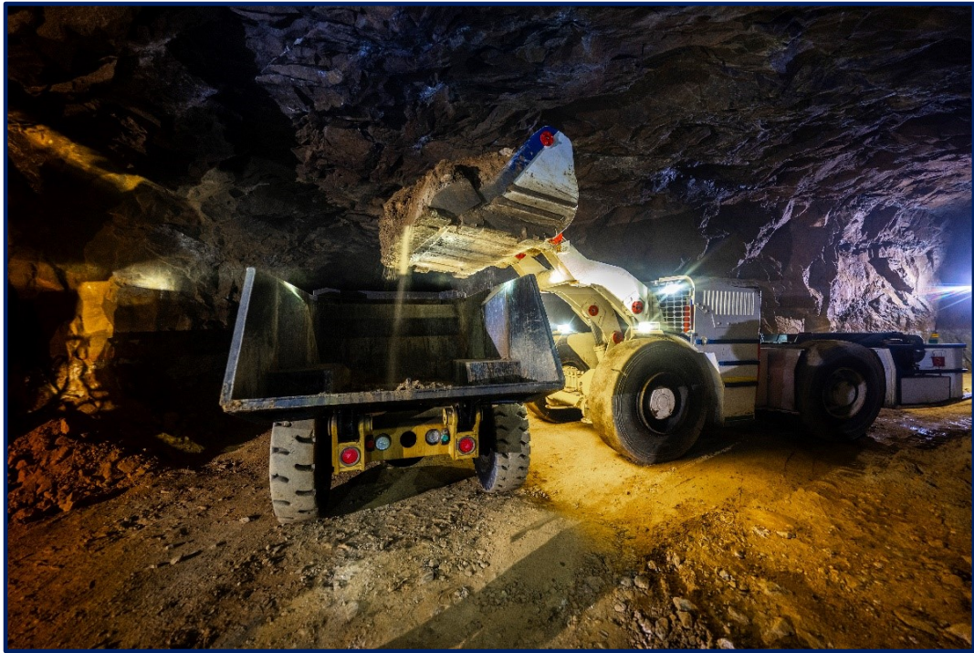
Photo 6: 143m Level draw point loading.
