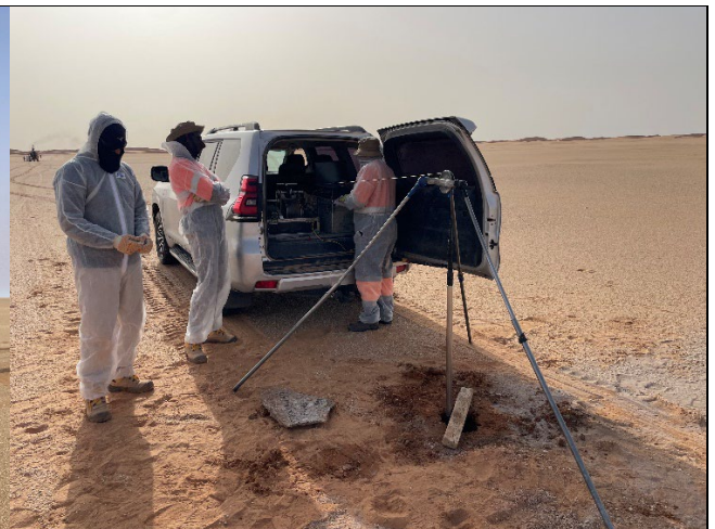
Downhole gamma survey at Sadi – Tiris
