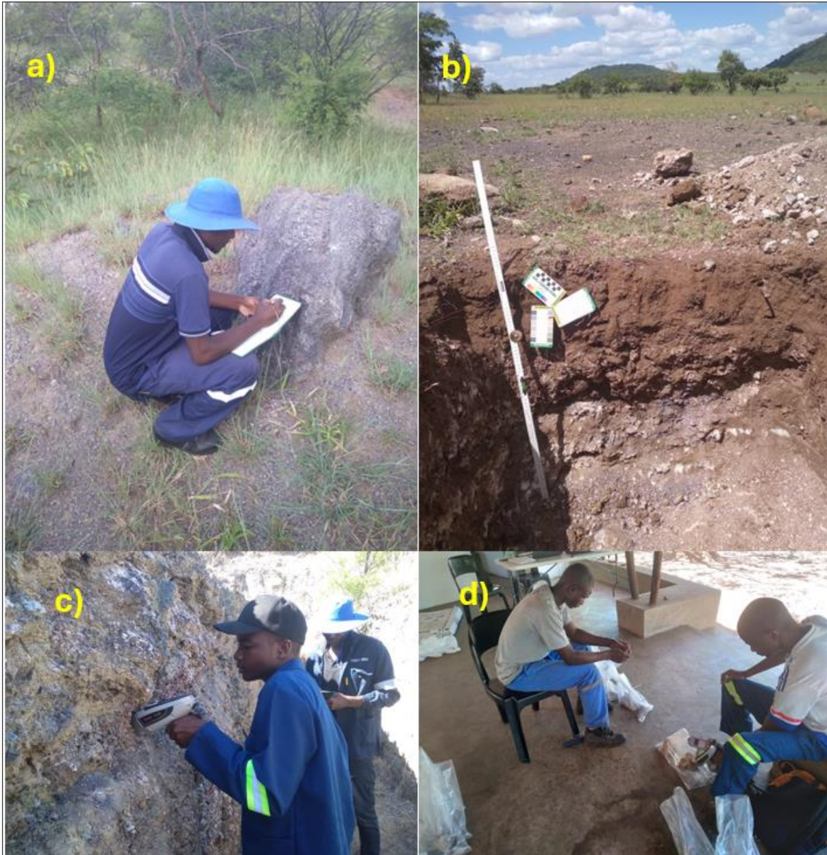
Figure 13: Images of exploration activities at Shawa. a) mapping taking place; b) pitting program to sample sub-crop during mapping; c) hand-held XRF analyses during field sampling and mapping; and d) hand-held XRF analyses at the sample handling facility of all rock and soil samples, with the rock samples to be analysed again by hand-held XRF after sample preparation (pulp samples).
