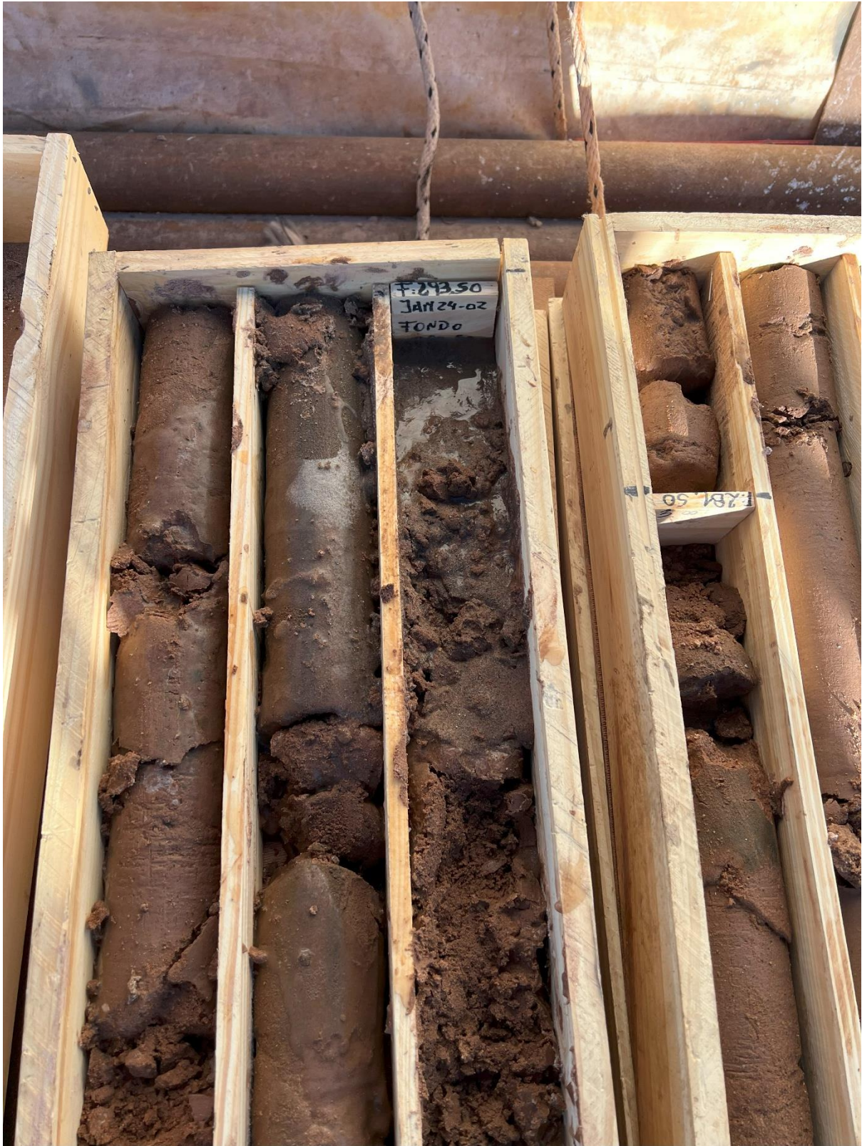
Figure 2. Wet drill core taken from 295m interval shows porous sands
