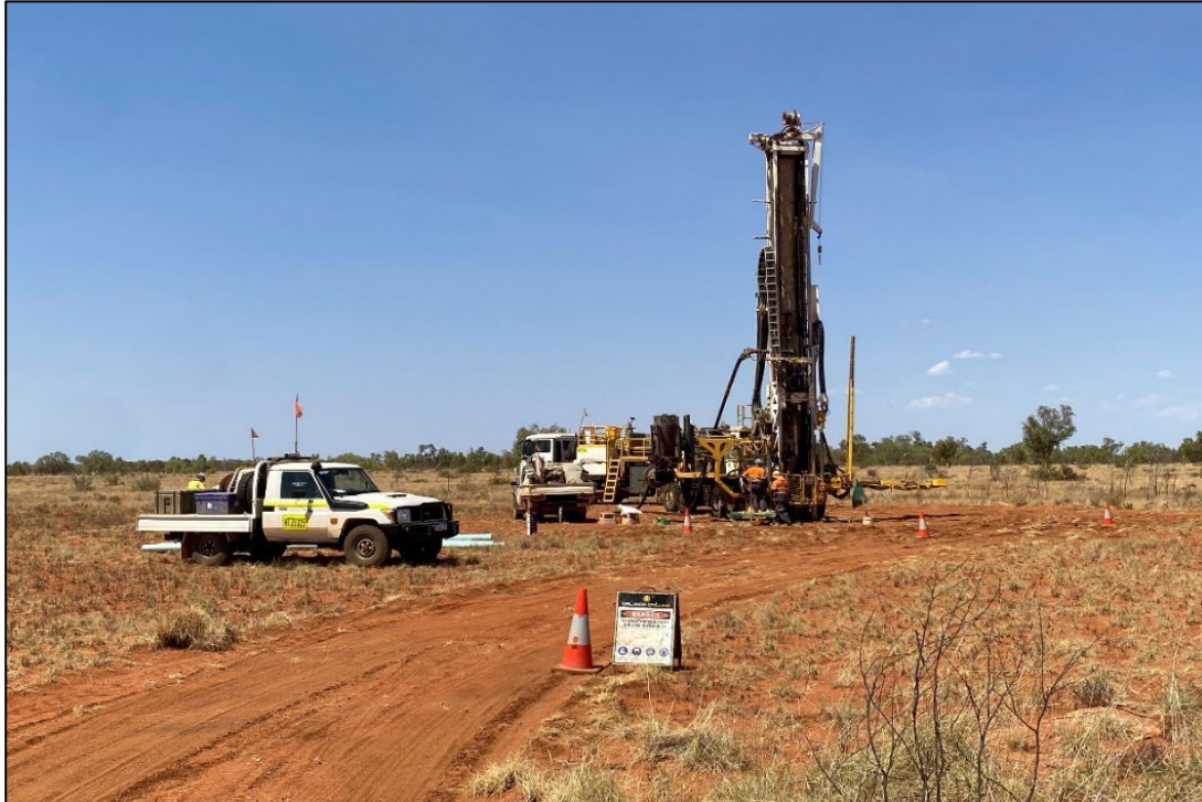
Figure 4. RC Drill Rig onsite at Quartz Hill.
