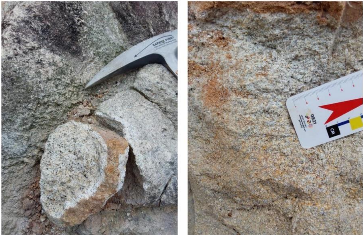
Figure 2. Fine to medium-grained equigranular tonalite composed of quartz, plagioclase, biotite and pyroxene/amphibole? with foliation on the edge of the pegmatites.
