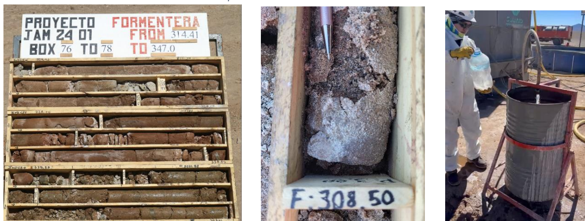
Figure 1. End of Hole showing porous sands and example at 308.5m, and 200L pump test
