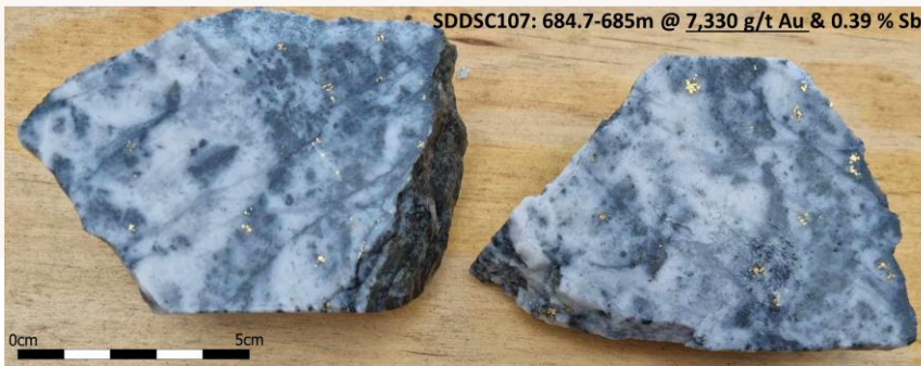
SDDSC107 from 684.7 m (within assayed interval 1.0 m @ 2319 g/t AuEq (2318.4 g/t Au, 0.3 % Sb) from 684.32 m to 685.35 m) showing cut core, with stibnite and quartz-carbonate veining with fine, disseminated frequent visible gold.
