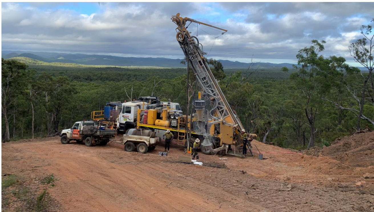
Figure 1 RC Drill Rig drilling ORR028 at Orient West ridgeline
