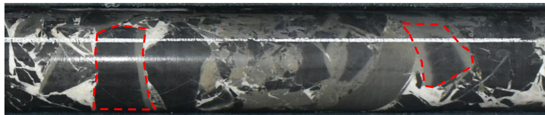
Dyke breccia with clasts displaying uniform & irregular alteration halos
