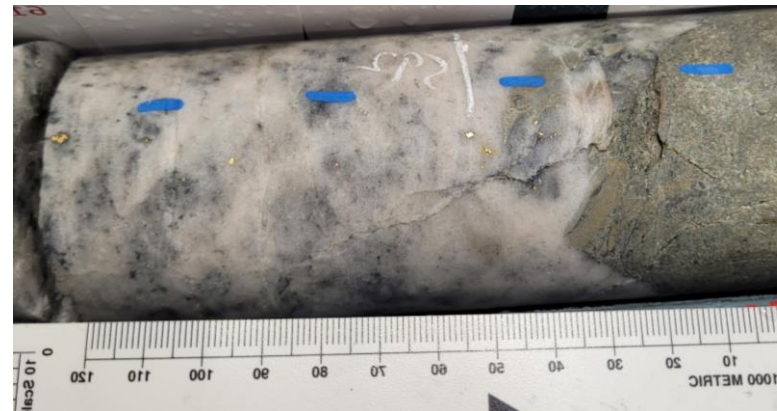
SDDSC082 from 592 m (within assayed interval 0.9 m @ 351.3 g/t AuEq (351.2 g/t Au, 0.0% Sb) from 591.4 m to 592.3 m) showing uncut core with quartz-carbonate massive vein with visible gold. mm scale
