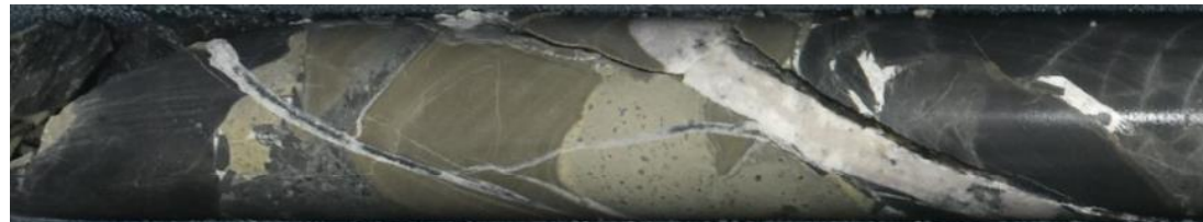
Overprinting relationship – Au Sb bearing Qtz veins overprint breccia
