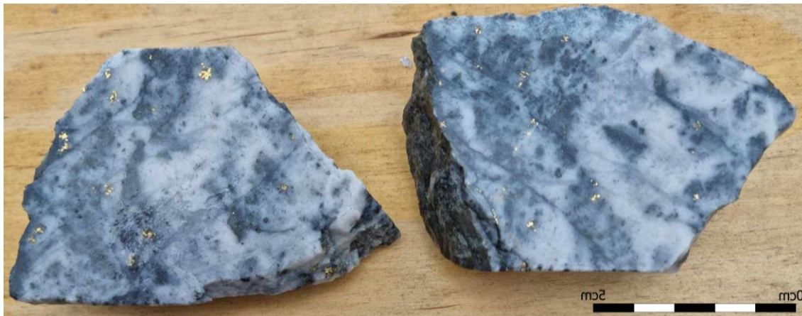
SDDSC107 from 684.7 m (within assayed interval 1.03 m @ 2319 g/t AuEq (2318.4 g/t Au, 0.3 % Sb) from 684.32 m to 685.35 m) showing cut core, with stibnite and quartz-carbonate veining with fine, disseminated frequent visible gold.
