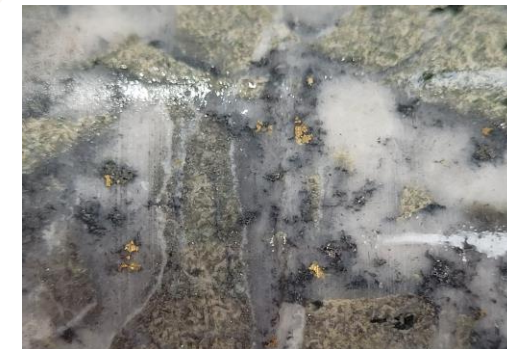
SDDSC077B from 739.9 m (0.8 m @ 1,741.5 g/t AuEq (1,736.4 g/t Au, 3.3% Sb) showing quartz-carbonate stockwork with visible gold, stibnite and sulphosalts in an altered dyke. Millimetre scale.
