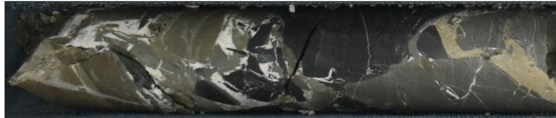
Mixture of dyke and qtz matrix surround altered & unaltered sediment clasts
