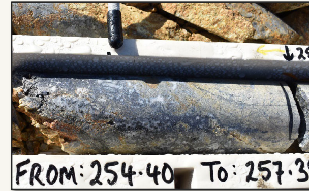
256.9m – Banded quartz, yellow-red sphalerite, galena, and MnO after rhodochrosite. 0.5m @ 1270g/t Ag, 2.58g/t Au, 10.05% Pb, 11.45% Zn
