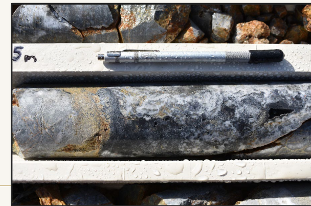
259.5m – Banded quartz, yellow-red sphalerite, galena, and MnO after rhodochrosite. 1m @ 243g/t Ag, 0.54g/t Au, 7.03% Pb, 14.65% Zn
