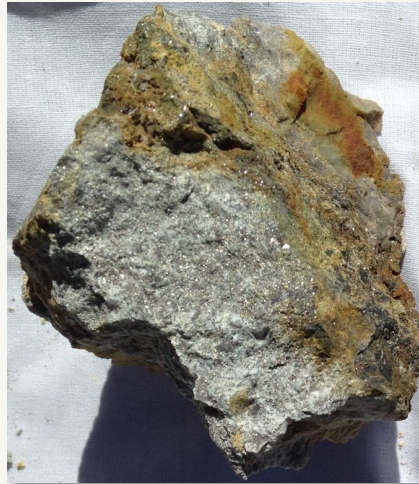
493g/t Ag , 0.44g/t Au, 1.12% Pb. "Waste" found on Mullock dump. Argillic altered, strongly sulphidic wall rock. EX455.
