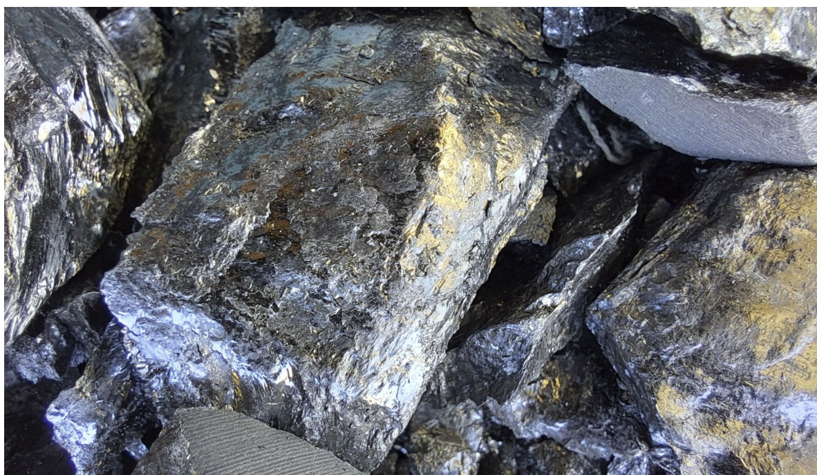
Figure 2: MI24DD01, 182.9m: High grade graphite in broken drill core.
