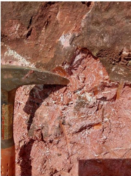
Figure 11. The fenitised Araxa shale in sample PL-066.
