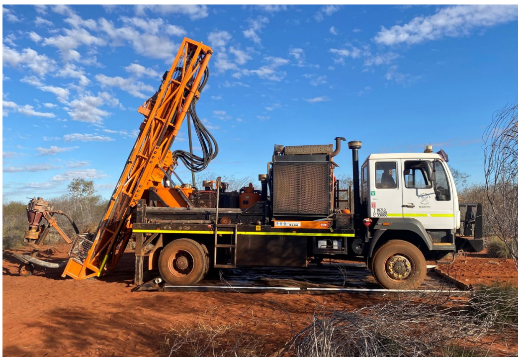
Figure 1: Air Core rig primed to drill NAE's first exploration hole at its Wagyu Gold Project
