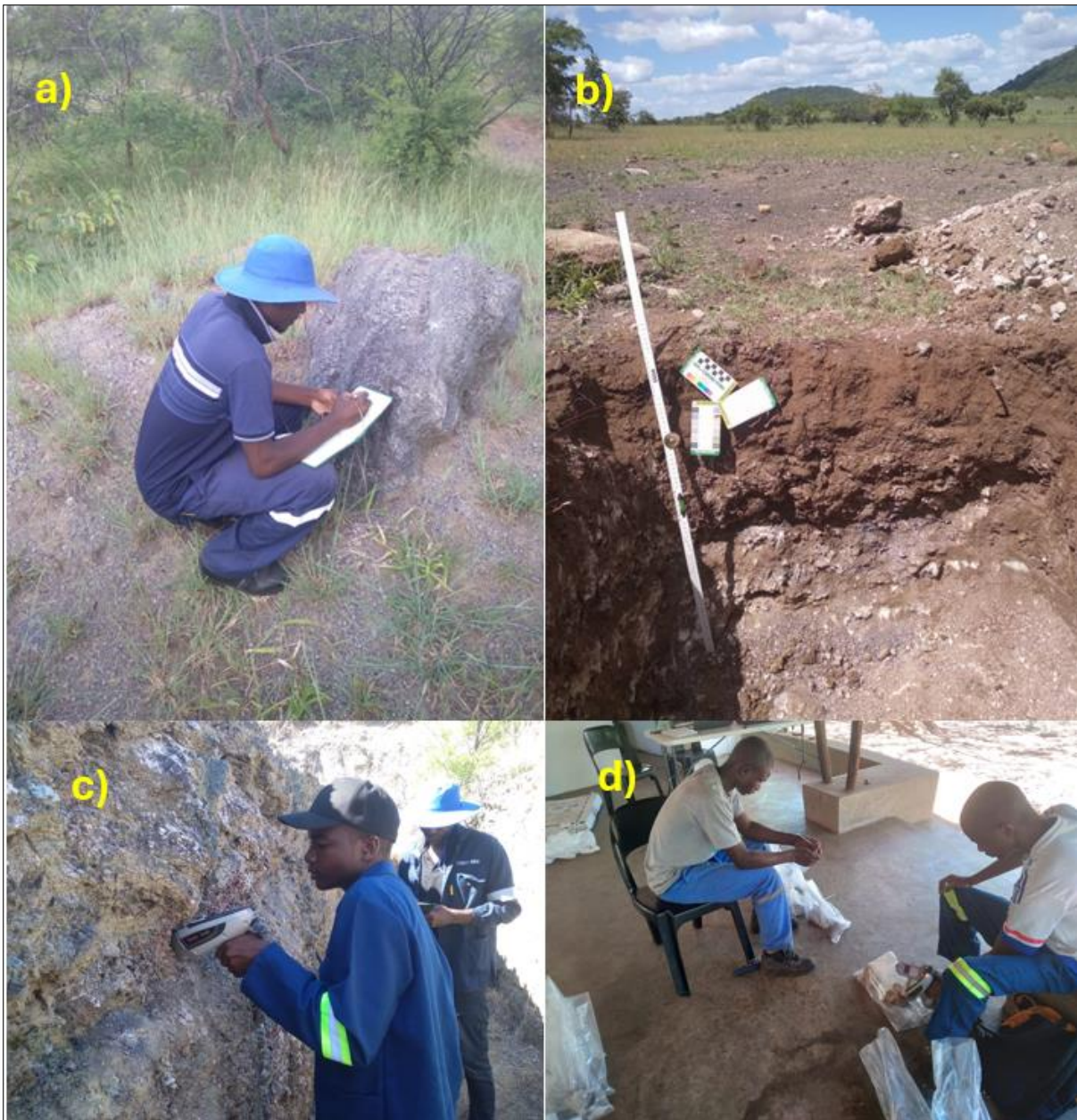
Figure 20: Images of exploration activities at Shawa. a) mapping taking place; b) pitting program to sample sub-crop during mapping; c) hand-held XRF analyses during field sampling and mapping; and d) hand-held XRF analyses at the sample handling facility of all rock and soil samples, with the rock samples to be analysed again by hand-held XRF after sample preparation (pulp samples).
