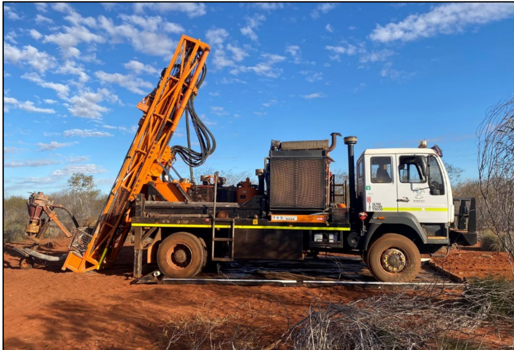
Figure 7: Air Core rig primed to drill NAE's first exploration hole at its Wagyu Gold Project.
