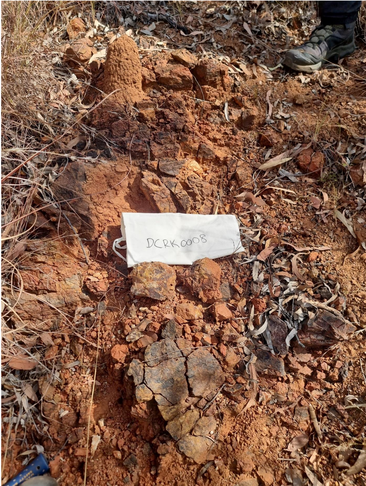
Deadman Creek Rock Chip (DCRK) 0008: Strongly hematite altered, brecciated and propylitically altered rhyolite, with iron rich (oxidised sulphide) veinlet stockwork.
