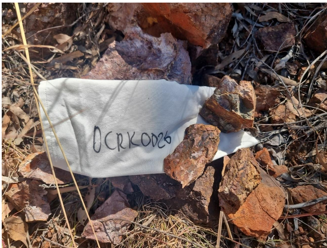
Deadman Creek Rock Chip (DCRK) 0026: Fractured rhyolite with pervasive haematite-limonite alteration plus 2mm wide goethitic veinlets
