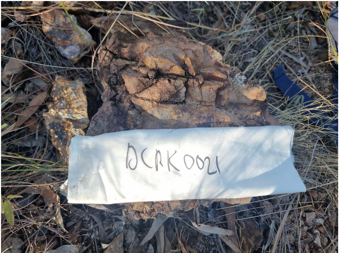
Deadman Creek Rock Chip (DCRK) 0021: Fractured and moderately propylitically altered rhyolite with 2mm wide goethitic veinlets
