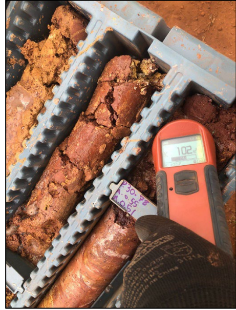
Figure 5: Magnetic susceptibility test for highly magnetised kamafugite stratigraphy
