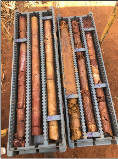
Figure 3: Significant intersection of Mineralised zone within kamafugite of Patos formation
