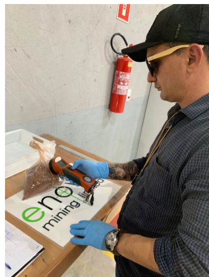
Figure 4: Magnetic susceptibility test for highly magnetised kamafugite samples
