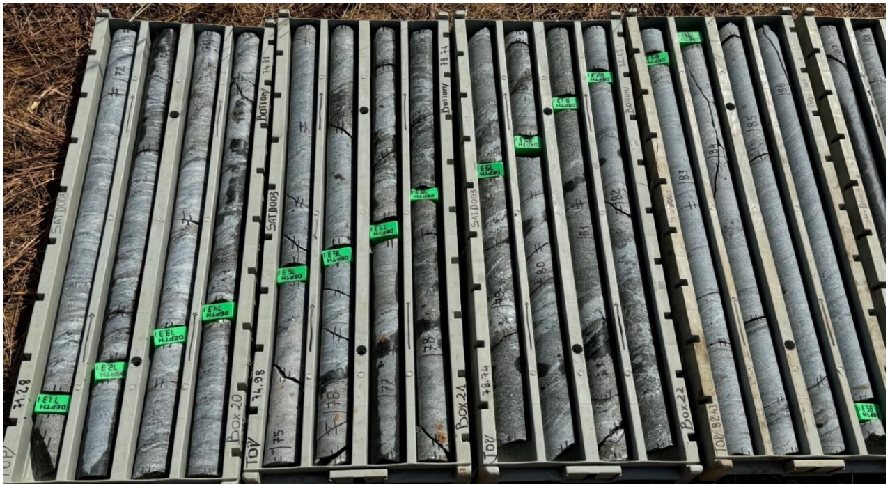
Figure 5. Drill core from drill hole SATD03 showing possible fine disseminated mineralisation at depth.
