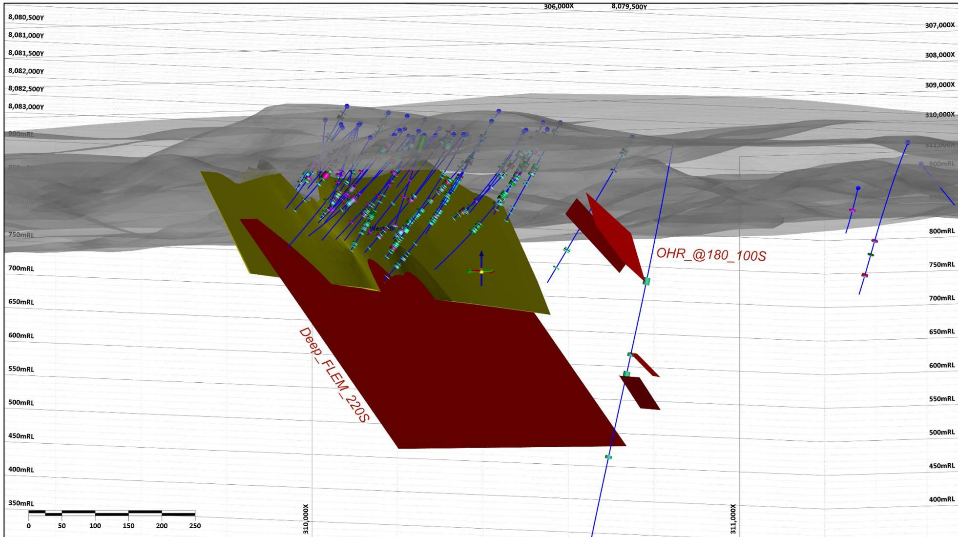
Figure 5 EM plate models with Drone magnetics model iso surfaces. 12500nT and 5000nT isosurfaces are shown
