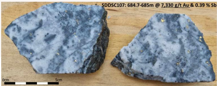
SDDSC107 from 684.7 m within assayed interval 1.0 m @ 2319 g/t AuEq (2318.4 g/t Au, 0.3 % Sb)
