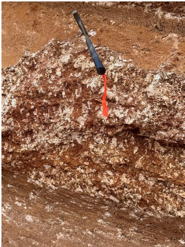
In-situ clay-rich saprolite at Area B
