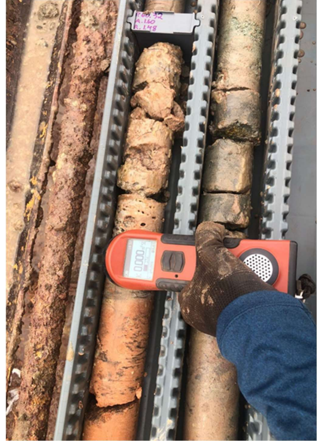
Figure 2: Magnetic susceptibility test on drill cores.
