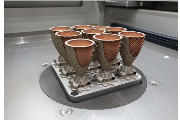
Powder bed fusion (PBF) rocket nozzles, MetalAM
