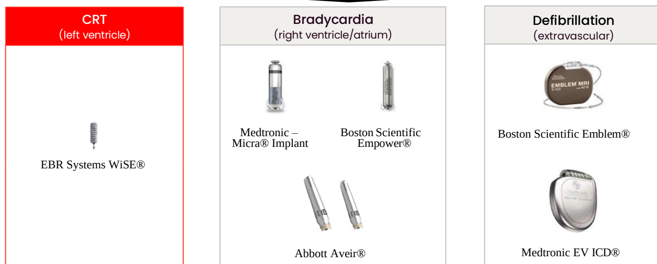
Figure 1.10: Current Leadless Pacemakers for Cardiac Pacing*
