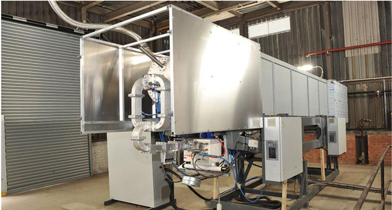
Figure 6: MPI Microwave Rotary Furnace (Source: [www.mpiuk.com](http://www.mpiuk.com) )
