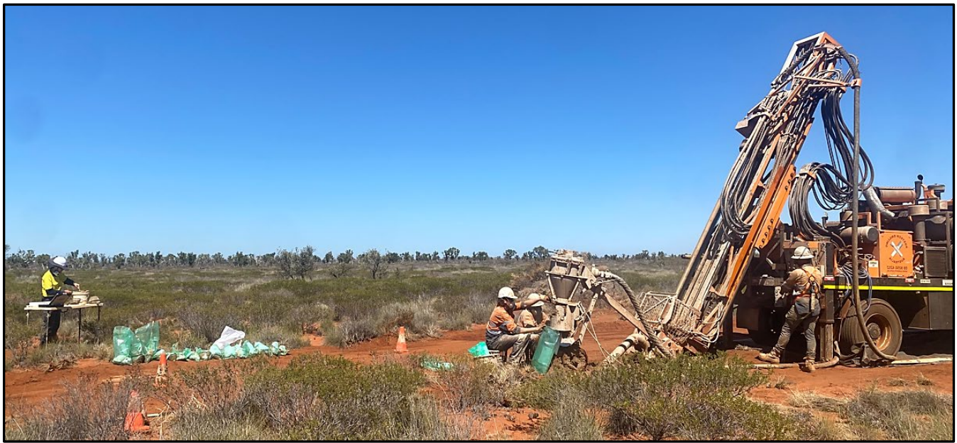
Figure 1: Air Core rig completing an exploration hole on Phase 1 at NAE's Wagyu Gold Project
