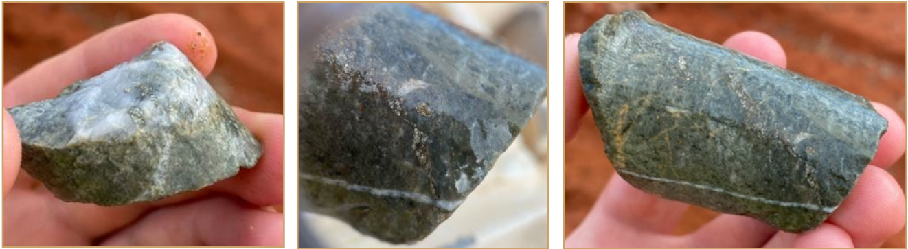
Figure 6: Intermediate intrusive rock (diorite) with sulphides from drillhole 24WA107, 39-40 metres, Target 6. The interval reported grades of 1.55 g/t tonne gold, 2.3 g/t silver, and arsenic of 119 ppm.
