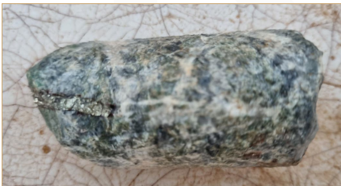
Figure 5: Sample from 71 to 72 m depth, 7 cm in length. Drillhole 24WA205. Hornblendes identified typical of Intermediate intrusive rock (diorite) with sulphides. Chlorite alteration associated late-stage quartz carbonate veining.
