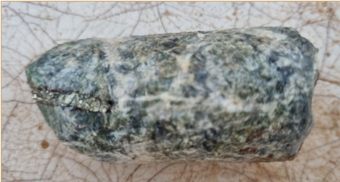
Figure 6: Sample from between 71 and 72 m depth, 7 cm in length, from drillhole 24WA205. Hornblendes identified are typical of intermediate intrusive rock; diorite. Sulphides are present. Chlorite alteration is likely associated late-stage quartz-carbonate veining.
