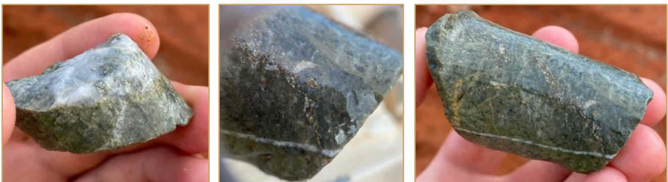
Figure 2: Intermediate intrusive rock (diorite) with sulphides from drillhole 24WA107, 39-40 metres, Target 6. The interval reported grades of 1.55 g/t tonne gold, 2.3 g/t silver, and arsenic of 119 ppm. ( See ASX Announcement 1 st Oct 2024 )
