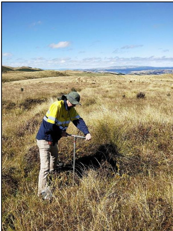
Figure 20 (a & b): Photos from recently completed field mapping and sampling work. (a) Soil sampling using a hand auger to get through glacial derived wind-blown cover (loess) and collect C horizon. (b) Historic test pit. NAE has mapped historic workings and test pits; these often provide additional outcrop/mineralisation information, rock chip samples and soil sample sites
