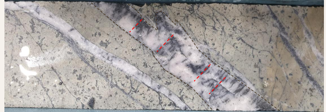
Quartz-carbonate-stibnite extension veins in altered dyke
