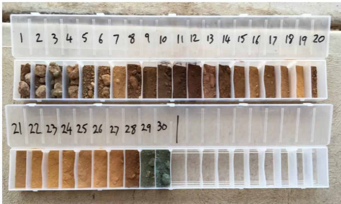
Figure 3: Chip tray for air core drill hole MA08 which intersected 9m @ 197ppm Sc from 8 metres including 3m @ 272ppm Sc from 13 metres. Numbers 1 – 30 on the chip tray denote individual downhole intervals (i.e., “10” means the drill sample obtained from 9 – 10 metres).
