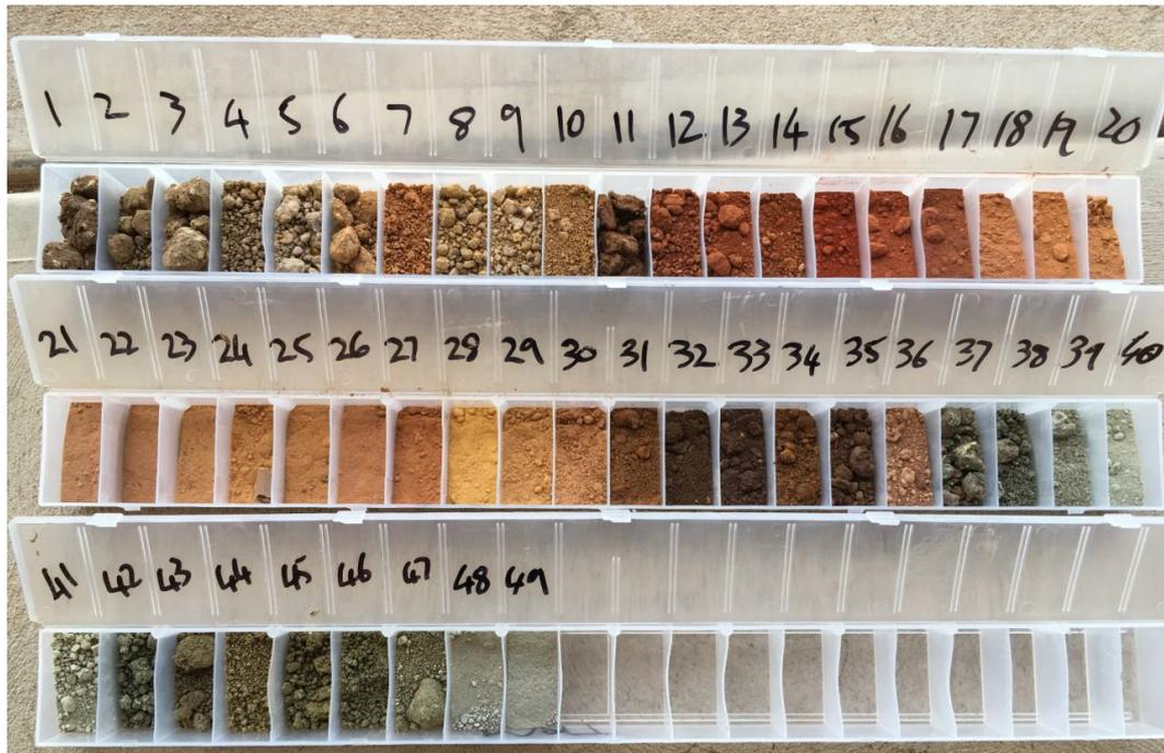
Figure 2: Chip tray for air core drill hole MA07 which intersected 18m @ 217ppm Sc from 30 metres including 6m @ 331ppm Sc from 31 metres. Numbers 1 – 49 on the chip tray denote individual downhole intervals (i.e., “10” means the drill sample obtained from 9 – 10 metres).
