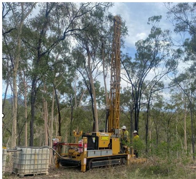
Figure 1 – Dart owned Alton Diamond drill rig on site at the Triumph Gold Project
