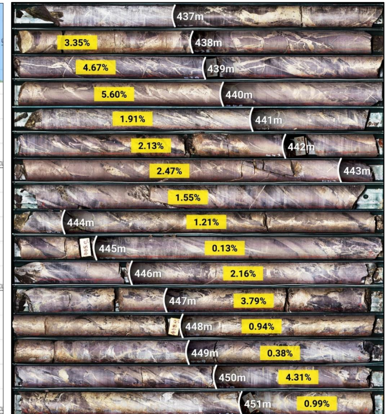
Diamond drill core from Severn hole ZS166 from approximately 436.5m – 451.4m. Core shows multi-stage pyrite-pyrrhotite-arsenopyrite vein network emplaced into strongly chloritized volcanoclastic sediments of the Crimson Creek Formation. Sn assays are shown in yellow as % Sn and depth intervals downhole in metres shown in white.
