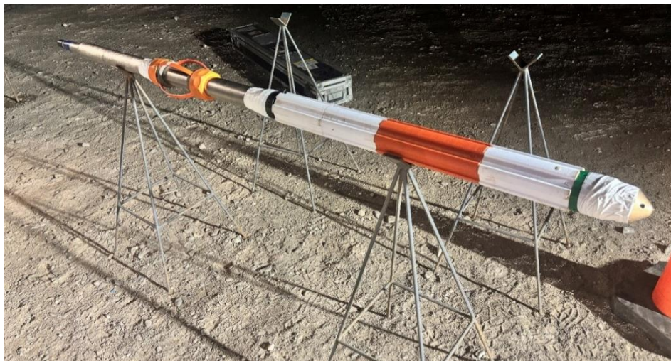
Figure 2. Borehole Nuclear Magnetic resonance tool being prepared.
