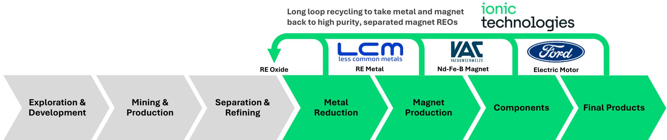
Ionic Technologies Belfast Magnet Recycling Feasibility Study<sup>1</sup> designed for 1,200 tpa end-of-life (EOL) NdFeB magnet and swarf feedstock, producing 400 tpa separated magnet REOs
