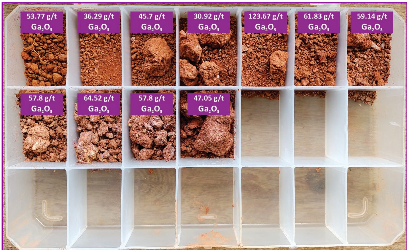
Figure 3 - CLD-AUG-109 auger core tray showing Ga 2 O 3 distribution over 1m intervals with exceptional 1m @ 124 g/t Ga 2 O 3 from 4m.
