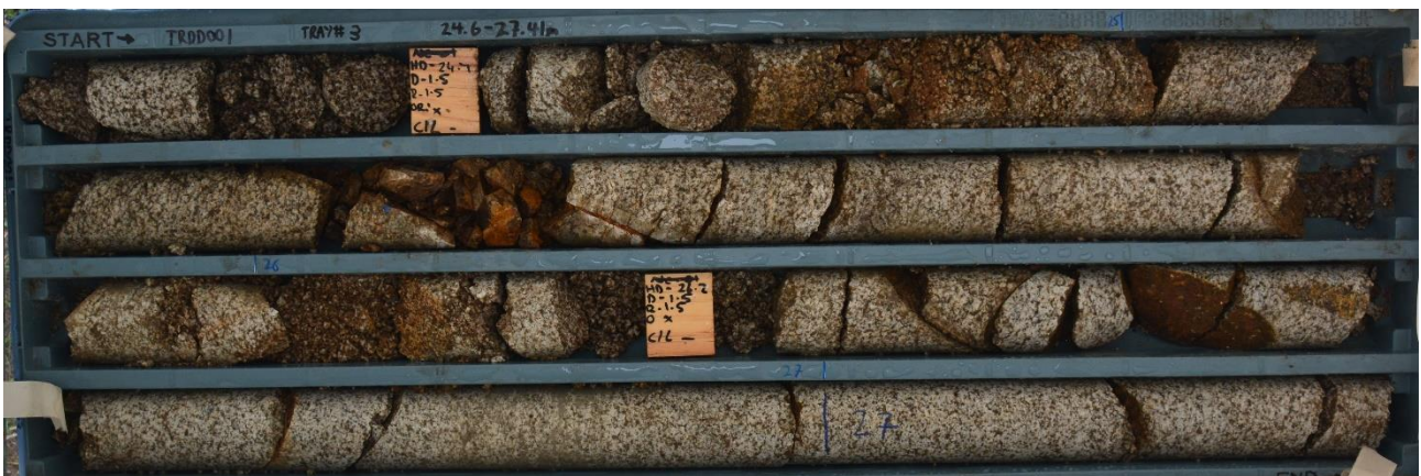
Figure 4: First competent core returned from hole TRDD001
