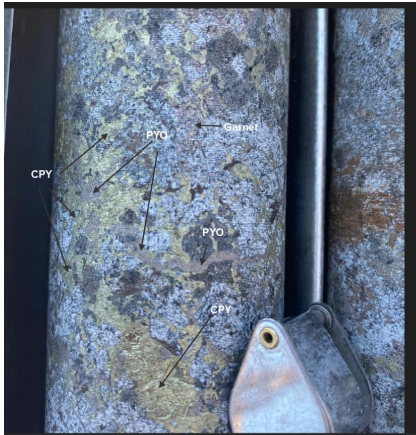
Figure 3: Copper sulphide mineralisation intersected within 608.00–609.00m interval in OFMSD083 with 2.69% copper and associated pyrrhotite and pyrite, which makes the mineralisation suitable for electrical geophysical methods.
