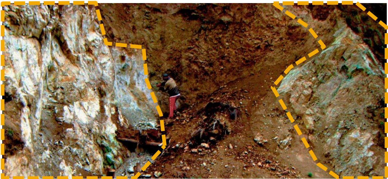
Figure 4: Historic sampling of felsic diorite porphyry outcrop with copper bearing malachite, at Venatica West showing cooling joints in contact with mineralised Breccia which returned 4.6% copper in sample 2253. Man is facing rock-chip sample site, orange outline shows outcropping sections of the porphyry which continues out of image.
